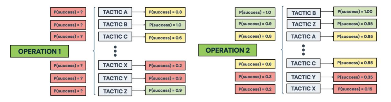
The results can be visualised better with secondary data collected from the planner's logs. In the first figure, the bayes planner begins with the atomic ordering (e.g. A-Z) as there is no data available. As the operation completes, the planner mathematically learns which abilities have the highest prospects of success.
